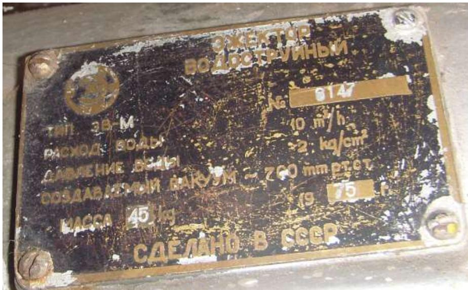
The ejectors are manufactured by Electrosila, and are equipment pertaining to generator Type TBB-200-2A;
