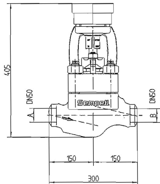
$$\begin{aligned} M_{d\ddot{o}} &= 40 \text{ Nm} \\ M_{dS} &= 30 \text{ Nm} \end{aligned}$$
